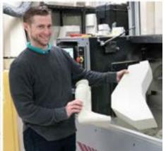
O & P technician, Richard Schloendorn, demonstrates how the new 3-Axis Carver cuts a mold from polyurethane foam in 10 minutes or less
